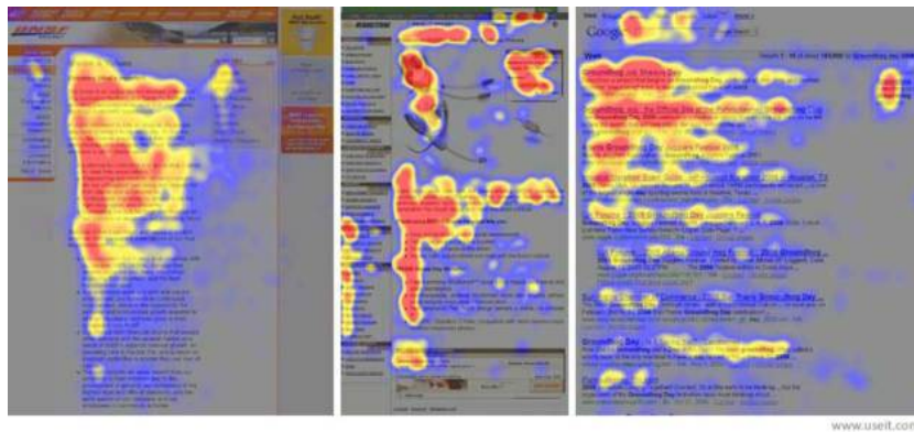
Figure 20. 'Heat maps' from user eye-tracking studies of three websites (18). The areas where users looked the most are coloured red; the yellow areas indicate fewer views, followed by the blue areas, which were the least viewed.
